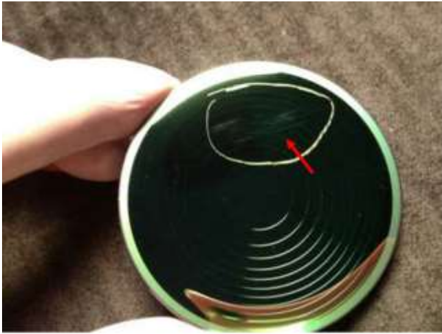
Scratches made by moderate abrasion followed the humidity test on real concave diffractive surface elements
