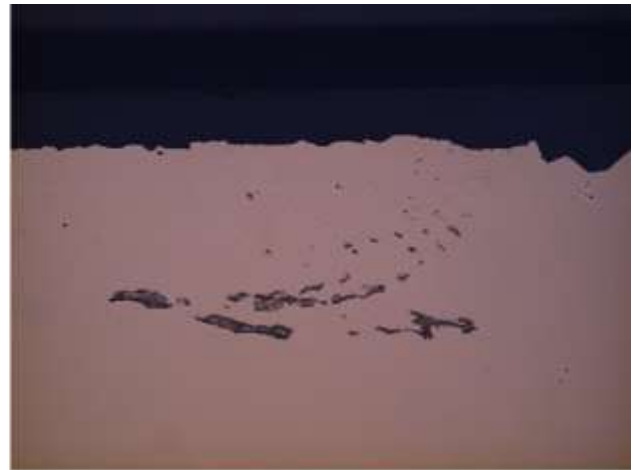
Peeling of coating on the edge of the element.
