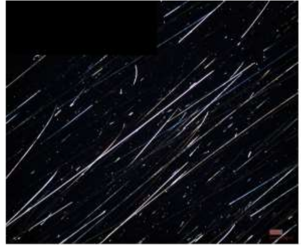
Scratches on the coating of copper coating mirror after moderate abrasion test (the same coating batch for the two mirrors)
