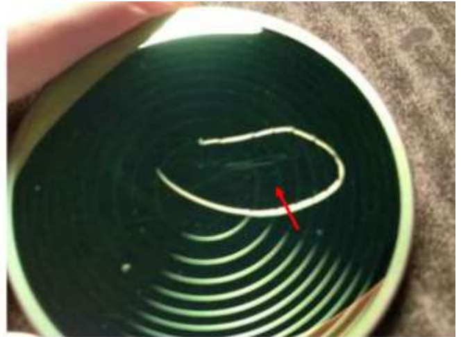
Scratches made by moderate abrasion followed the humidity test on real concave diffractive surface elements
