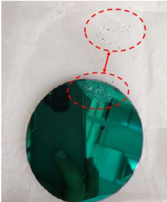
Disintegration of the coating of IR window, observed after opening the packaging
