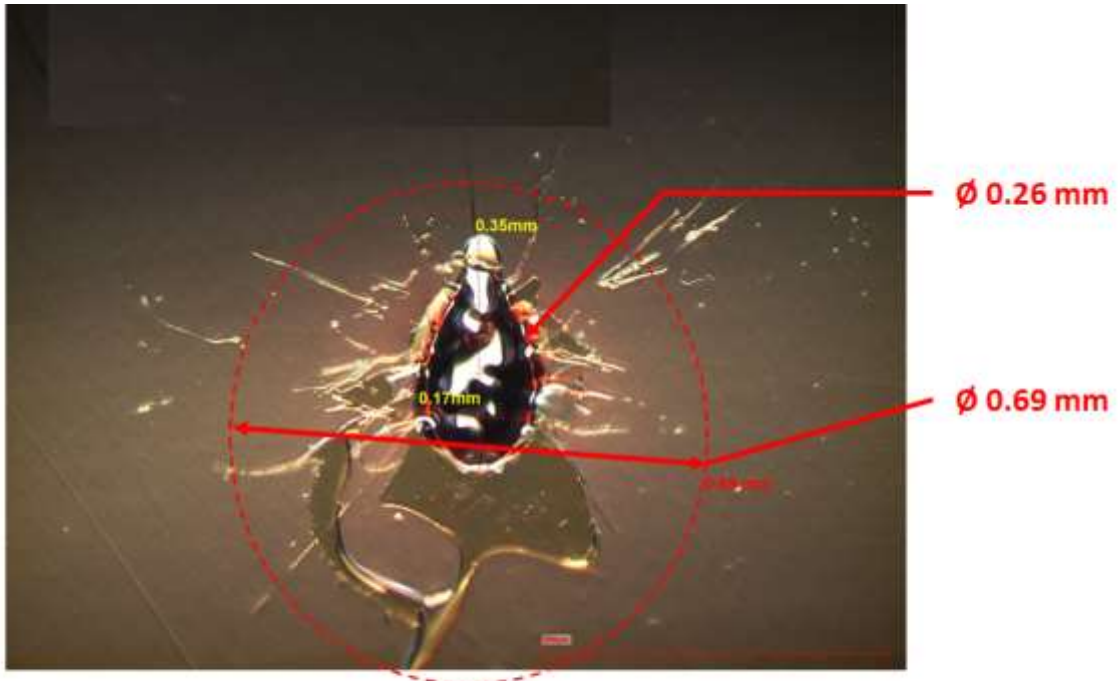
Deep dig with uplift of the IR coating, total of \varnothing 0.69 mm (the dig itself of \varnothing 0.26 mm).
