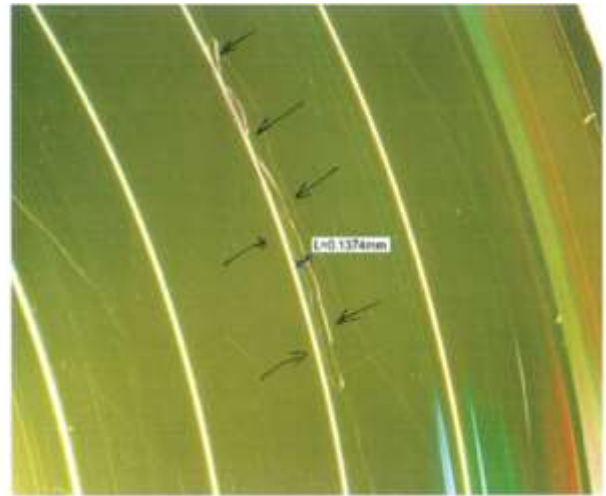
Peeling on IR coating of concave aspheric-diffractive surface, width of 0.1374 mm max.
